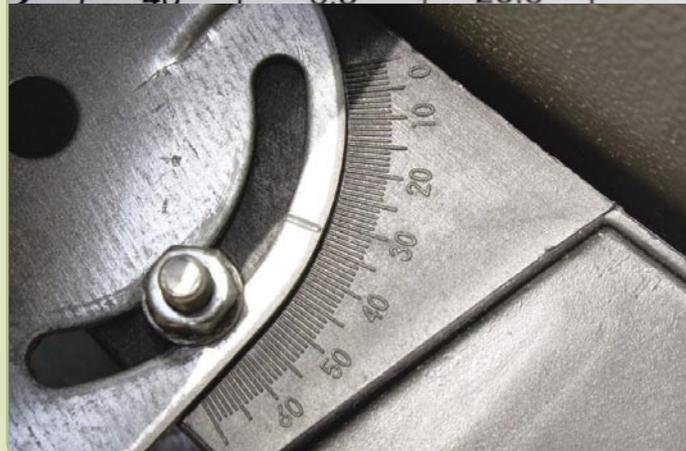
■ (Figure 3) Table Excerpt and Antenna Declination Scale
